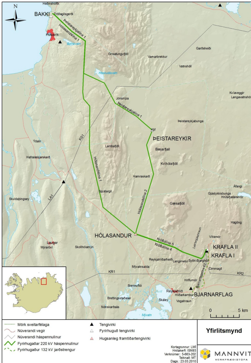
Figure 13: Layout of power transmission lines from geothermal areas in Northeast Iceland to the proposed industrial site at Bakki (Mannvit hf., 2010 b)
